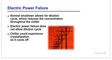
During normal shutdown, an absorption chiller goes through a dilution cycle to reduce the concentration of the solution throughout the chiller. At this reduced concentration, the chiller may cool off due to lower temperatures of the space surrounding the chiller, but it will not be in danger of crystallizing.
